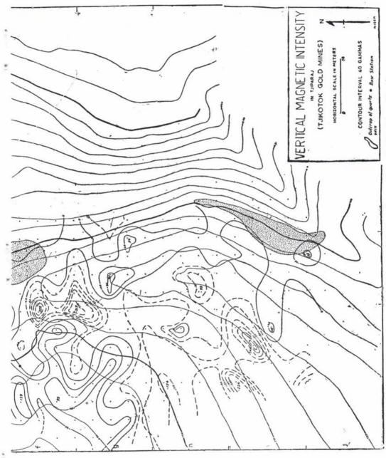
Fig. 3. Magnetic anomalies of vertical intensity at Tjiparaj, Tjikotok gold mine.
